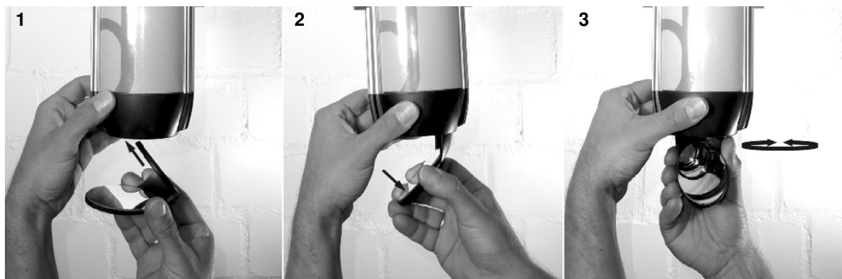
Fig. 9: Inserting the deflection mirror
