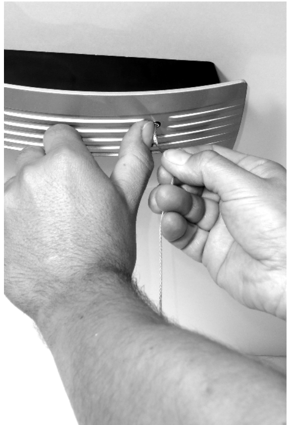
Fig. 7: Opening the cable tensioner
